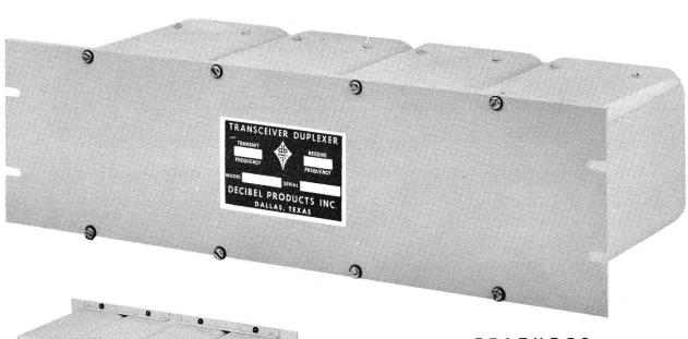
Models **DB-4075** and **DB-4076** are high performance, compact base station duplexers for use with stations operating in the 450-470 MHz, or 470-512 MHz bands. The models consist of quarter-wave coaxial cavities interconnected in a bandpass configuration with double shielded, teflon dielectric cable. A high quality tunable capacitor is used within each cavity to enhance the bandpass characteristics at the reject (undesired) frequency.
