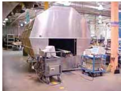
100% IM and Return Loss Testing On All Antennas
